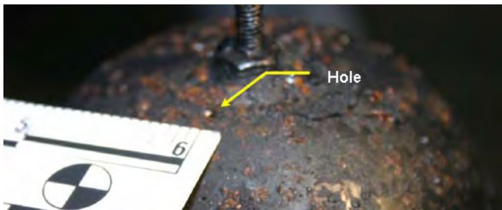
Figure S- 6. Close-up of LSH-5020 float, showing corrosion and hole
