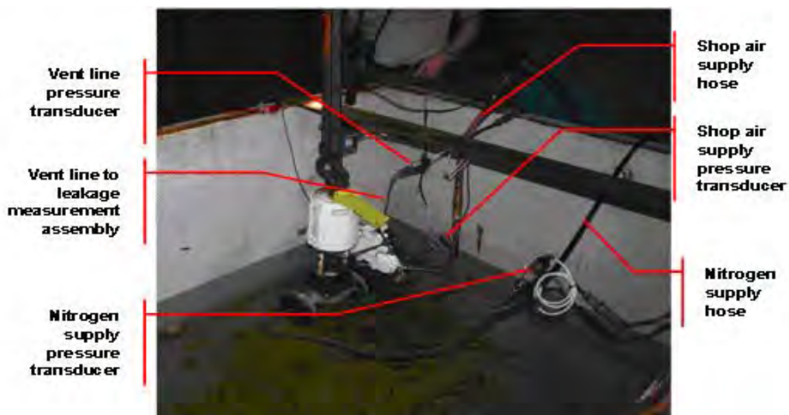
Figure S- 7. PCV-5002 shop testing
